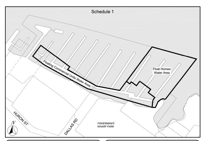
Beginning at Monument 7-1, thence on an azimuth of 317° 12' for a distance of 172.63 metres to the south-western corner of Lot A, Plan VIP73551, thence 36° 12' 10" for a distance of 44.75 metres, thence 126° 00' for a distance of 8.00 metres, thence 36° 00' for a distance of 11.00 metres, thence 126° 00' for a distance of 10.00 metres to the POINT OF COMMENCEMENT
