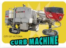
Have you ever poured melted chocolate into a mold and watched it set in place? The Curb Machine does that on our streets, pouring concrete curbs and gutters of all shapes and sizes to keep vehicles on the road
