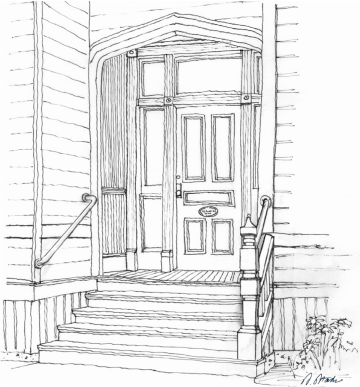
Heritage Consultant Stuart Stark's design for a code compliant railing on 1139 Burdett Street, which uses a simple pipe rail extending from the house to the newel post.
