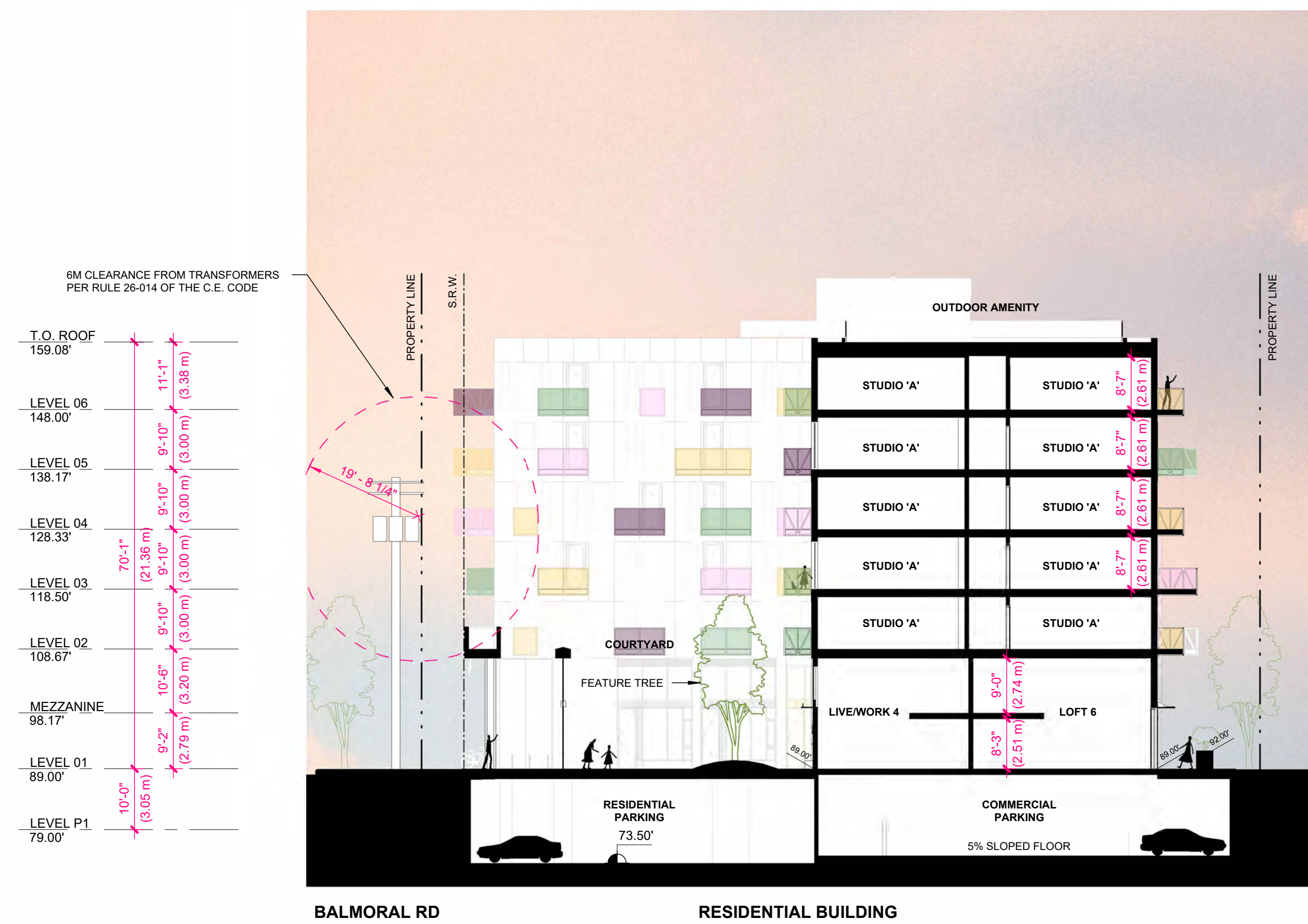
2 SITE SECTION THROUGH RESIDENTIAL COURTYARD LOOKING WEST
