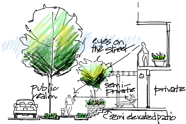
Diagram showing incorporation of entries to individual ground floor units that are accessible and clearly visible from the fronting street.
