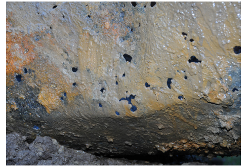
Corroded underground oil tank.
