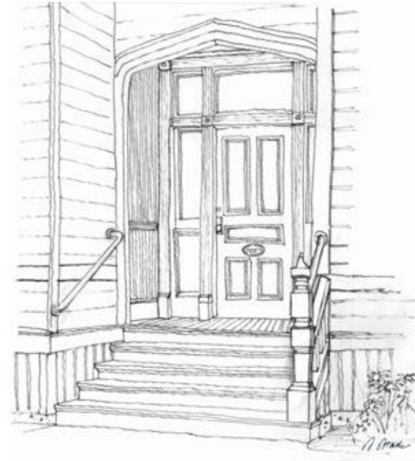
Heritage Consultant Stuart Stark's design for a code compliant railing on 1139 Burdett Street, which uses a simple pipe rail extending from the house to the newel post
