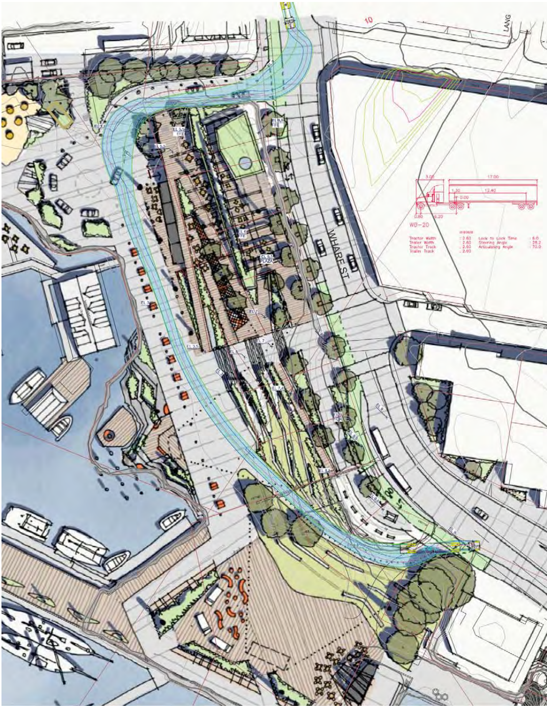
Exhibit 1.3 WB-20 Loading Truck Turn Paths
