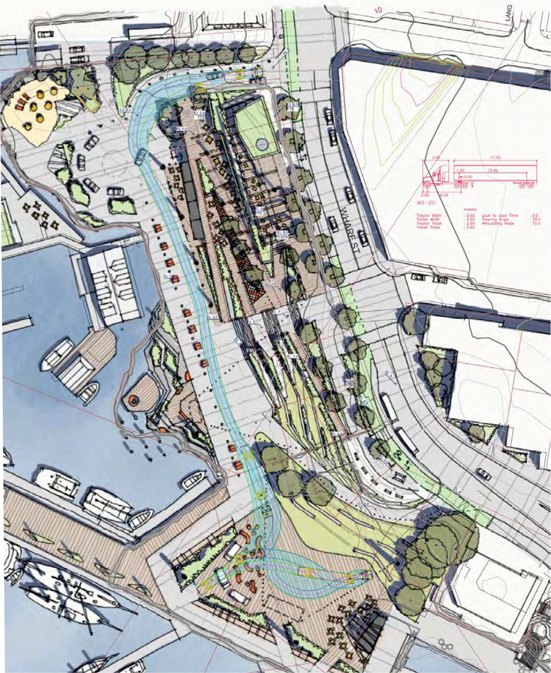
Exhibit 1.4 WB-20 Loading Truck Alternative Turn Paths
